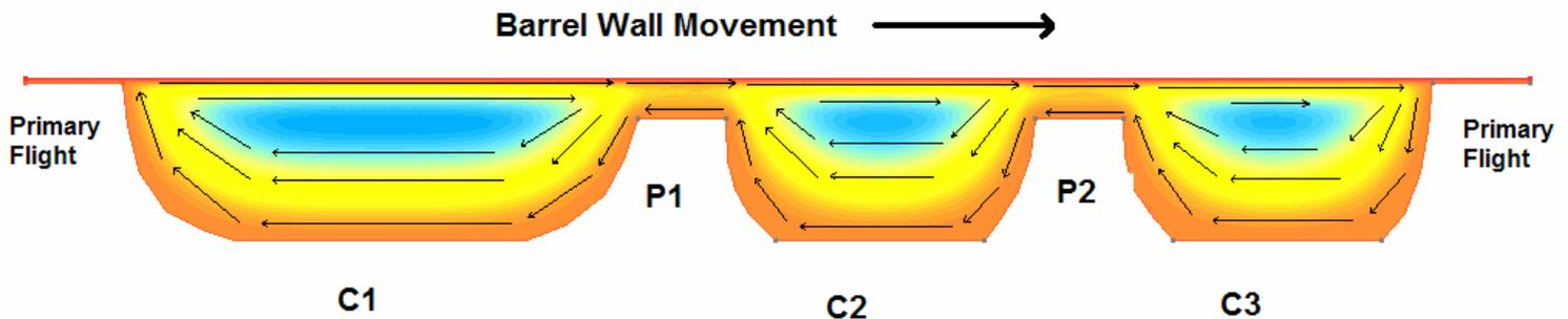
**Figure 12.** Pump areas between C2 and C3 showing back flow
