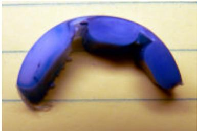
**Fig. 9: One inch Cross Section of Extrudate Between Screw and Breaker Plate**
