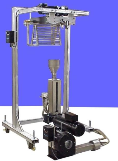
RCP-0750 Microtruder with 1 inch die fixed height take-off.
