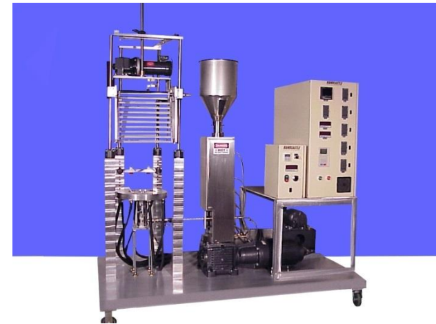
RCP-1250 Microtruder with 2.0 inch die integrated platform and adjustable height take-off.
