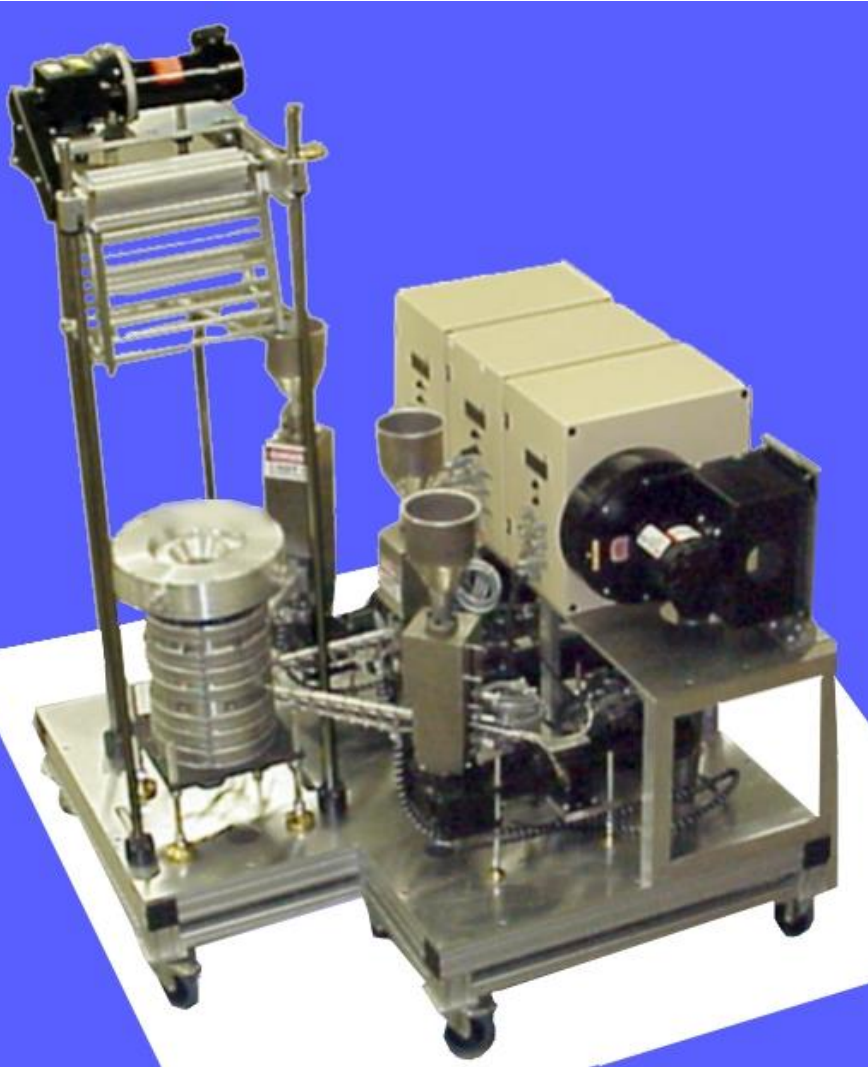
Three RCP-0750 Microtruders for ABCBA structures with adjustable height take up.
