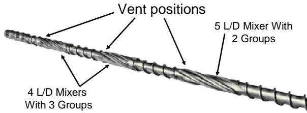
A "Group" is composed of the sequence of channels and pumps such as for this study, C1, P1, C2, P2, C3. Each group is axially bound by a flighted clearance.
