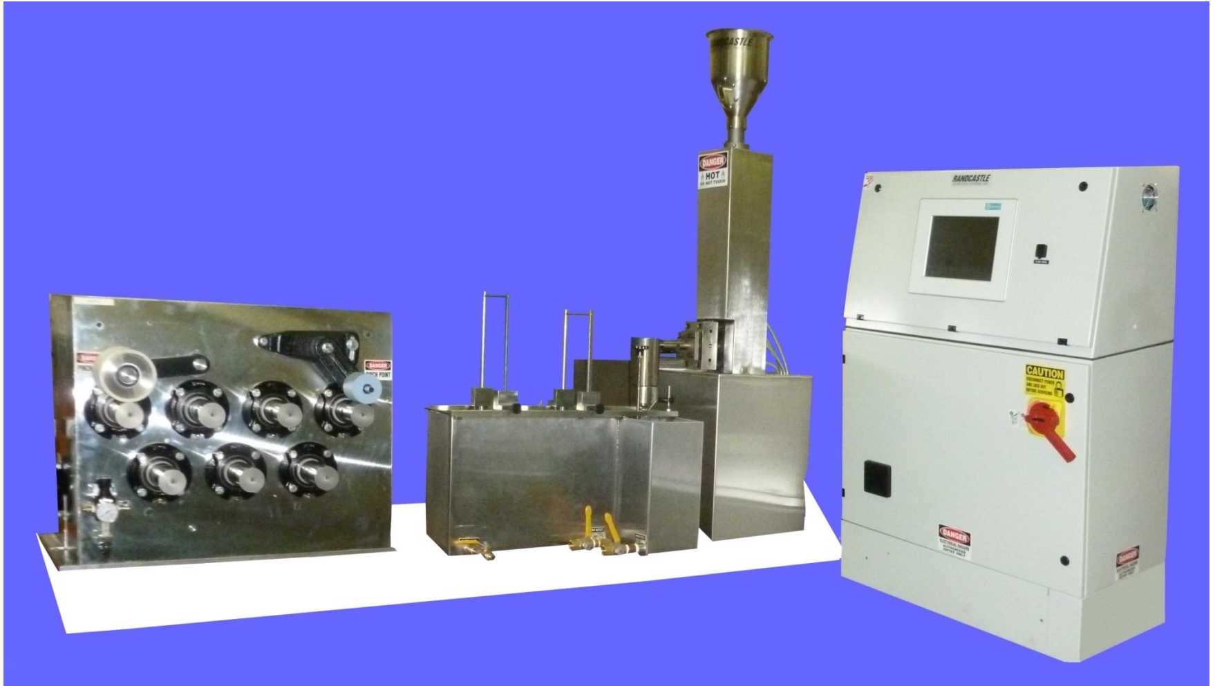
Closer View of First Part of Line: PLC, RCP-0750 Extruder, Stainless Steel Die, Stainless Steel Vertical Water Bath and First Godet With Stainless Steel Rolls
