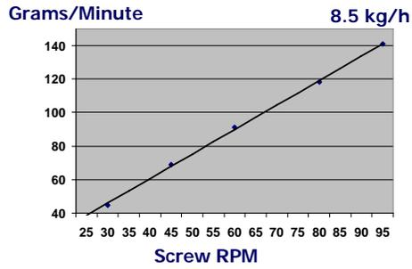
**Figure 7. – Graph of RPVC Pellet Output on 1 Inch Extruder**
