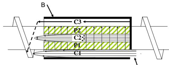
Upstream flow eliminated by increasing the input flow.
