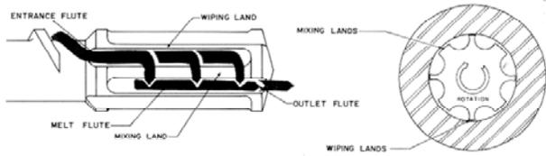
The entrance flute dead ends at the wiping land. Pressure, generated upstream, forces material over the mixing flute where the material is sheared. The higher the pressure, the higher the heat generation.
