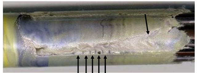
These appear to be partially melted pellets
